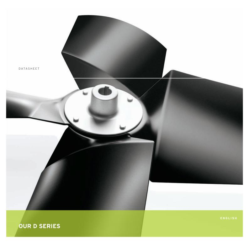
The D series covers diameters from 400mm up to 660mm. The relatively small diameter and the broad, paddle-shaped profile of the fan blades makes the D series ideal for smaller heat exchanger applications such as oil coolers, air-cooled condensers and dry coolers. With fan blades of glass reinforced polyamide it can be used in low temperature evaporator applications as well.
