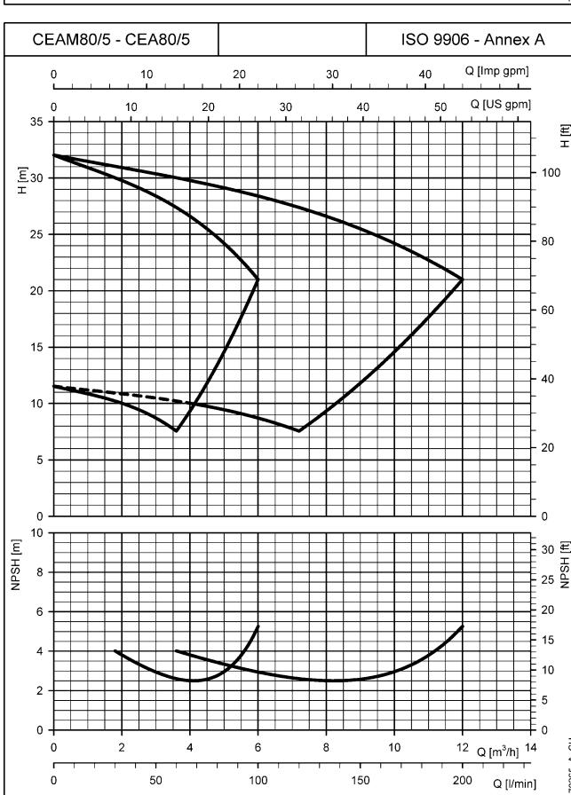
The performance curves do not take into account flow resistance in the valves and piping.
