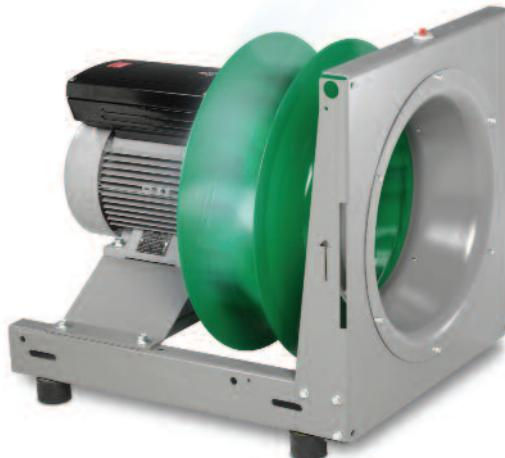
The integral motors are 3-phase motors with integrated frequency converter. No separate motor cable between the frequency converter and the motor is needed because the frequency converter is mounted on the motor. An EMC filter is built into the frequency converter. Integral motors are well suited for fan operation due to the low level of sound that they generate.
