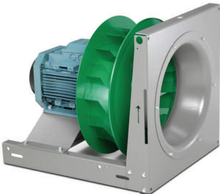
The direct driven CENTRIFLOW Plus plug fans are available in 17 sizes and cover airflows up to 25 m<sup>3</sup>/s and pressure rises up to 2300 Pa. CENTRIFLOW Plus is characterized by high efficiency. The impeller has backward curved blades. The CENTRIFLOW Plus is available in two versions, standard and ATEX (sizes 022-100)
