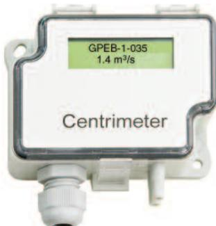
CENTRIMETER provides a simple and accurate means of measuring a fan's airflow. The measuring device is self-calibrating and automatically sets a reference zero point and adjusts itself for changes in ambient temperature. The device allows the user to select the displayed units of measured airflow, either in  $\text{m}^3/\text{s}$  or  $\text{m}^3/\text{h}$ , or differential pressure in Pa.
